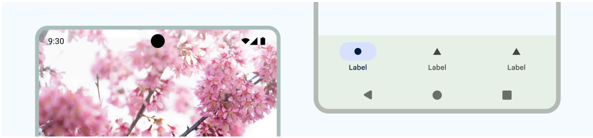
Figure 8: Transparent bars using the edge-to-edge feature , ideal for letting your content shine through using the most screen space.
